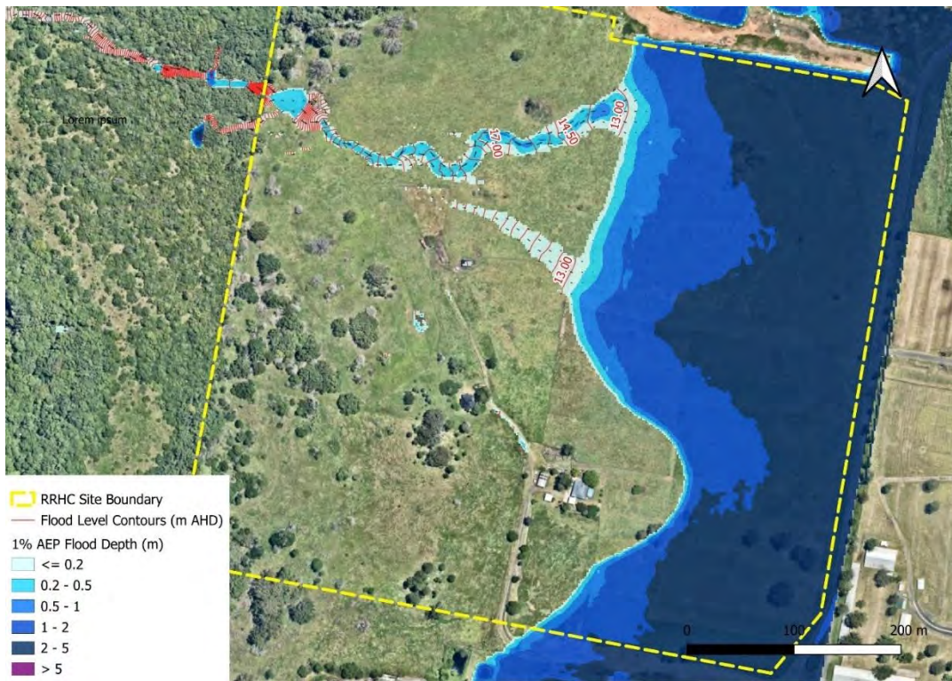
Appendix B 7: 1% AEP flood depths and levels at the proposed RRHC site under existing site conditions
