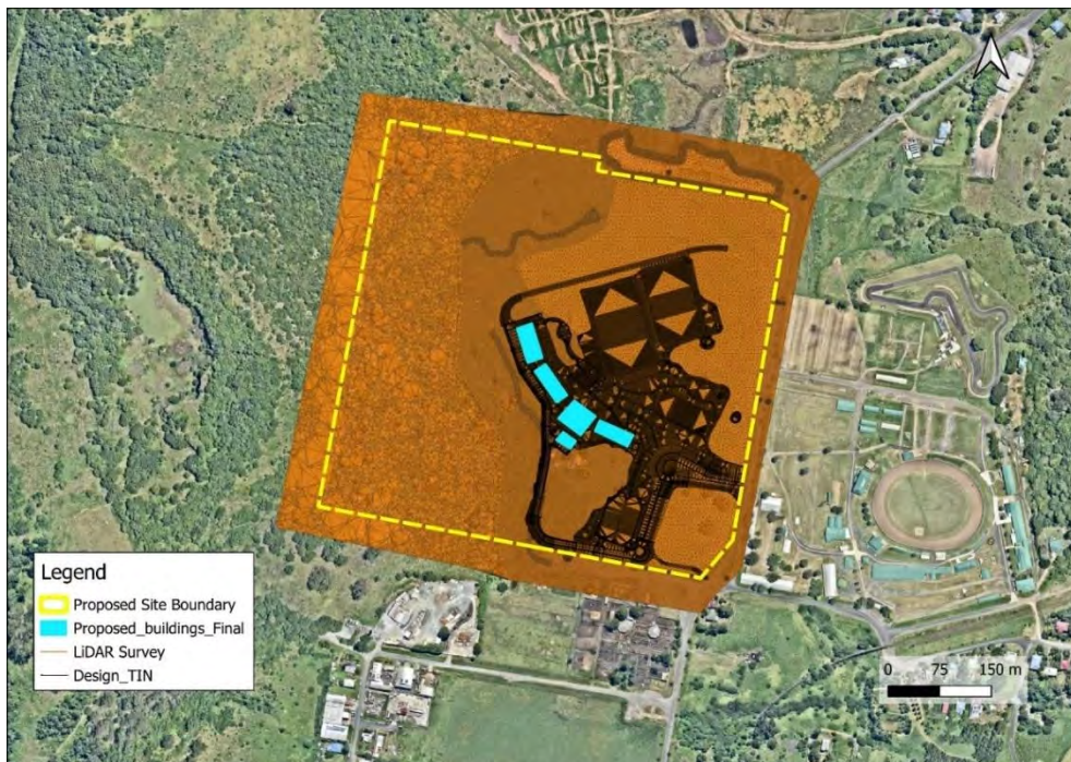
Figure 13: Design TIN used for the post-development model
