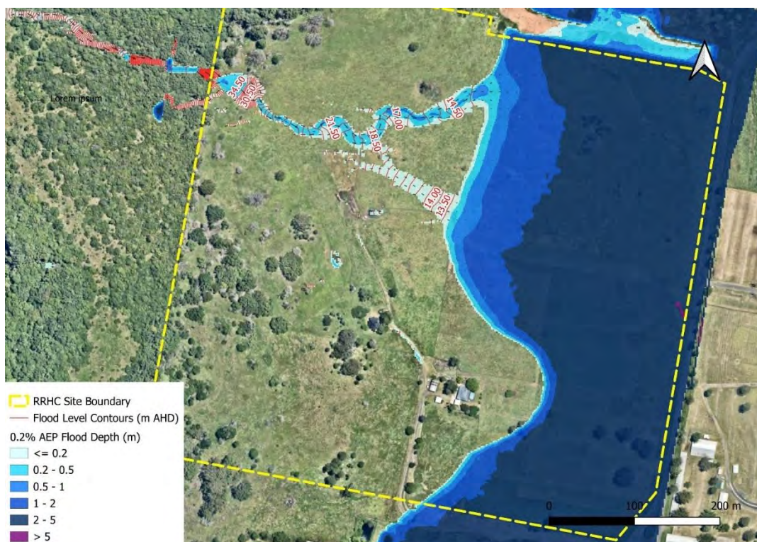
Appendix B 10: 0.2% AEP flood depths and levels at the proposed RRHC site under existing site conditions
