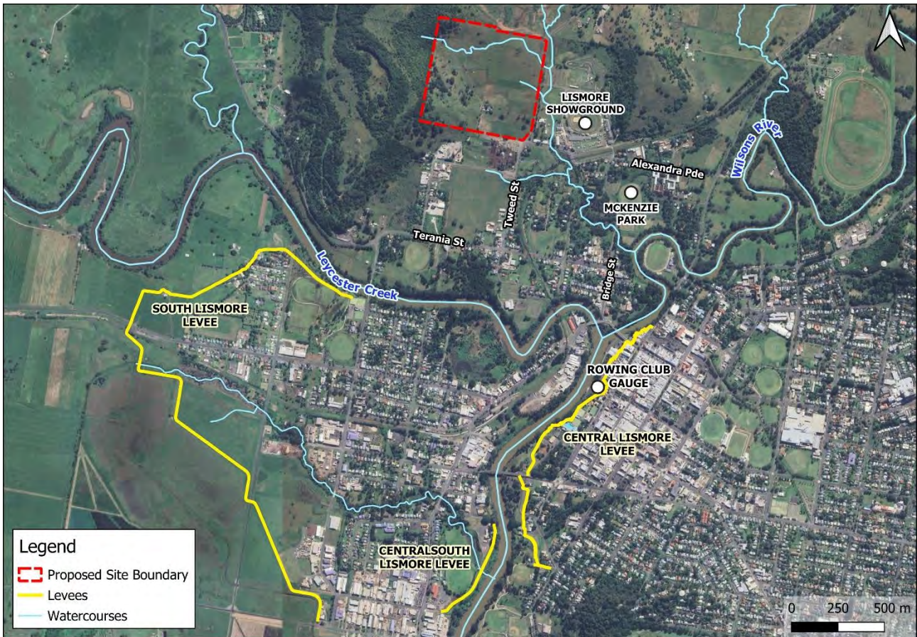
Figure 4: Hydraulic controls in the vicinity of the site
